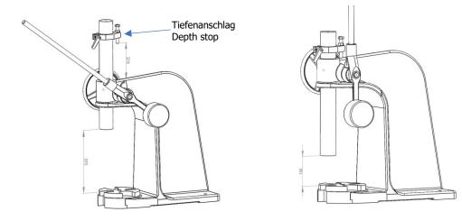
After altering the position of the depth stop and initial operation the clamping lever and the counter nut of the adjusting screw <u>must</u> both be tested for stability to prevent unintentional and uncontrolled movement of the press or part of the press.
