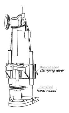
After the table is adjusted into position, it must again be secured with the clamping lever.
